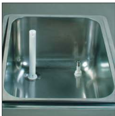
Refrigerated tank where the temperature of the mix is constantly checked by a thermometer.
