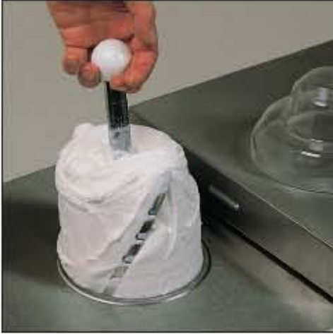
Vertical BEATER which can be easily removed to extract the ice cream.
