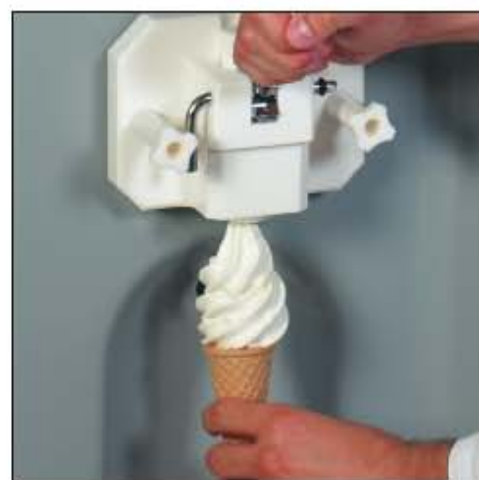
Distribution tap for fast dispensing of ice cream cones and cups. A protective top is available (optional) that can be removed when serving the ice cream.
