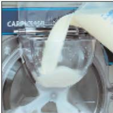
Wide loading hopper with safe lid to pour the mix into the machine.
